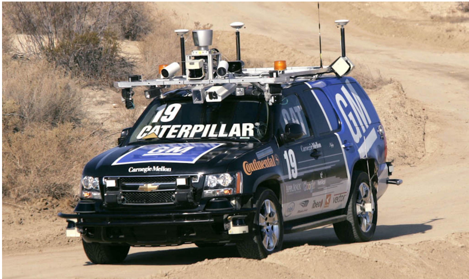
Figure 1.1: The autonomous Chevy Tahoe, 2007 DARPA Urban Challenge winner, Carnegie Mellon University[1][2]
